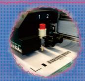
The plotter uses the barcode information to find the correct cut data from the USB memory stick and cut it. This eliminates human error.
