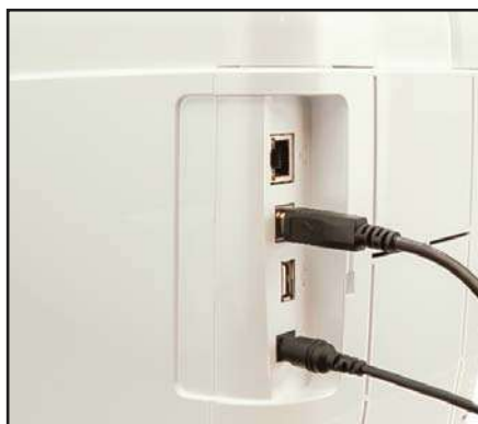
Interfata USB2.0 (high speed), inclus in 10/100 ethernet, Wi-Fi (optional)
